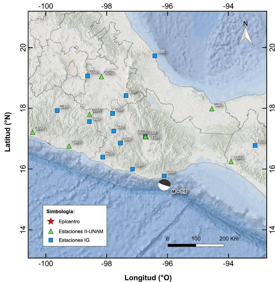
**Figure 1.** The epicenter of the M 7.5 23 June 2020 earthquake and seismic stations that recorded the event. The stations belonging to the Accelerographic Network of the National University of Mexico's Engineering Institute (RA-IIUNAM) are operated by the Seismic Instrumentation Unit (labeled *Estaciones II-UNAM*). The stations operated by the National Seismological Service are labeled *Estaciones IG*.
