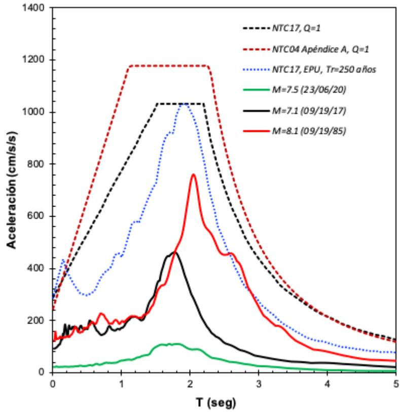
**Figure 6.** Comparison of design spectra, uniform hazard, and earthquake response spectra recorded at station SCT2.
