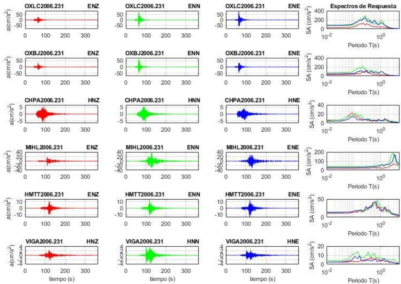
**Figure 4a.** Recorded accelerograms and estimated response spectra for records obtained during the earthquake of June 23, 2020 (M7.5)
