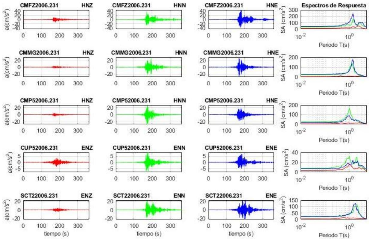
**Figure 4d.** Registered accelerograms and response spectra for records obtained during the June 23, 2020 (M7.5) earthquake.
