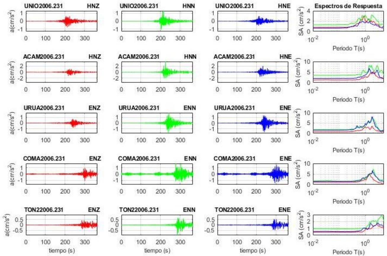
**Figure 4c.** Registered accelerograms and response spectra for records obtained during the June 23, 2020 (M7.5) earthquake.
