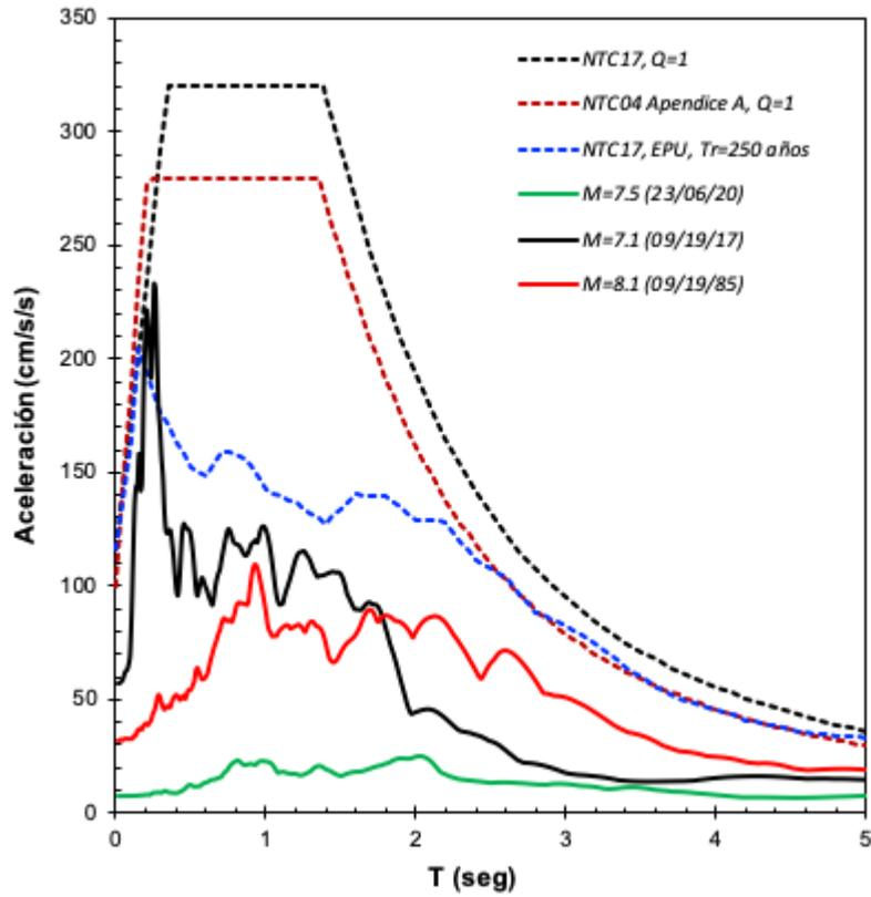
**Figure 5.** Comparison of design spectra, uniform hazard, and earthquake response spectra recorded at the CUP5 station.
